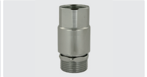
Chrome-plated brass. Backflow preventor according to DIN 19884 and DIN EN 1717. Avoids that cleaning agents come into the potable drink circuit in case of excess pressure in the water pipe. Required when direct connection to pump
