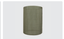
Complete with screen (stainless steel). 400 micron. Max. 10 bar / 60 l/min / 60 °C
