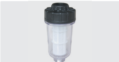
Complete with screen (plastic). 60 micron. Max. 10 bar / 50 l/min / 50 °C
