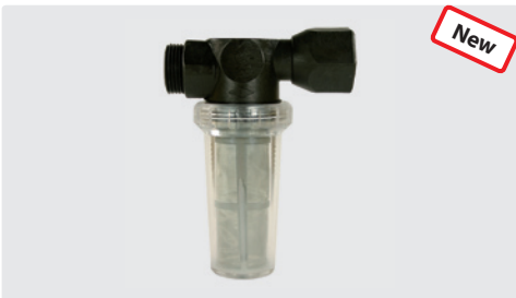
Complete with filter fine core washable (stainless steel and plastic). 50 microns. Max. 6 bar / 60 °C / 50 l/min
