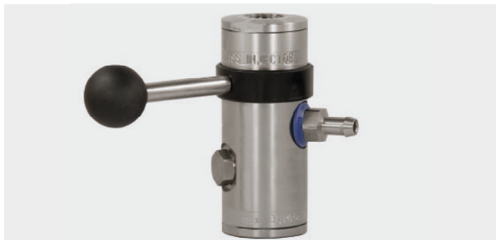
☞ 1/2" F - ☜ 1/2" F. Injector ST-167 with hose tail 9 mm. The chemical dosing is adjusted by 8 exchangeable nozzle inserts (0.5 - 2 mm). Max. 350 bar / 100 °C
