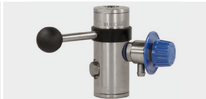
☞ 1/2" F - ☜ 1/2" F. Injector ST-167 with metering valve ST-161. Max. 350 bar / 100 °C
