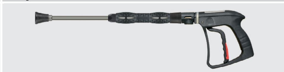
Professional steam gun. Lance 400 mm stainless steel with extension ST-9.1 220 mm and nozzle protector ST-12 without high pressure nozzle. Max. 20 bar / 200 °C
